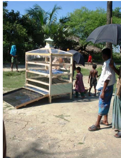
JOBS engage local carpenters to build solar driers to hygienically process dried fish
